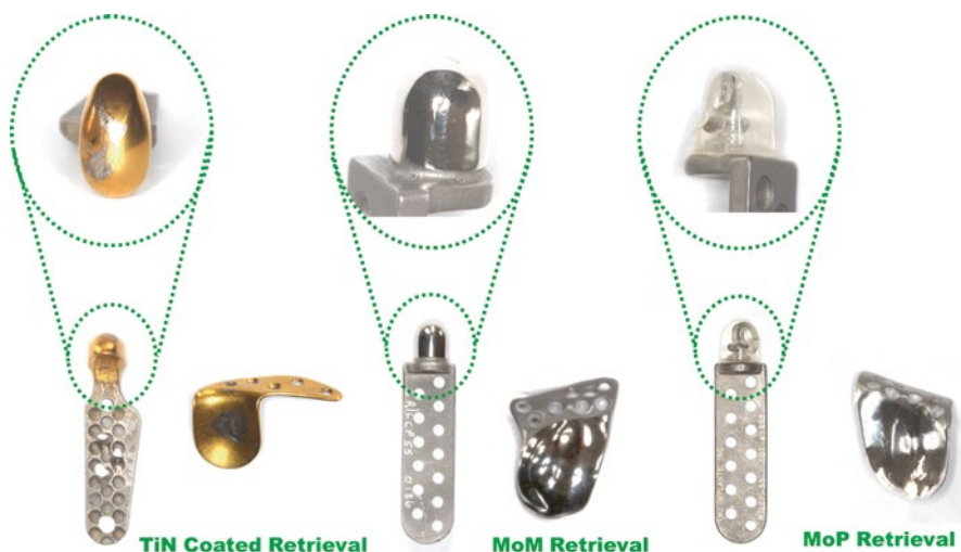
Fig. 10.6 Evidence of tribocorrosion from TMJ TJR implant surfaces
