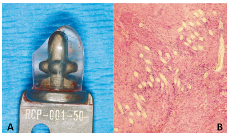
Fig. 3.5 (a) Polymethylmethacrylate (PMMA) head of a failed TMJ Inc. condylar component demonstrating wear 3 years after implantation. (b) Particles of PMMA demonstrated in the peri-articular tissue
